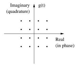
Here  $x_i$  and  $y_i$  are each permitted to have four levels per dimension. The 16-symbol QAM signal may be generated using a system of the following form:
