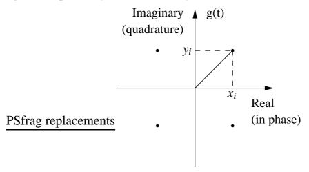
This case differs from the previous only in a shift in the carrier phase reference. This example of M-ary PSK where M=4 is called *quadrature* phase-shift-keyed (QPSK) signalling. The diagrams above are called the QPSK constellation diagrams, and contain information regarding the permitted values of the complex envelope.
