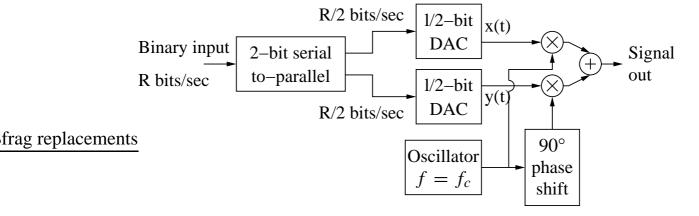
This scheme is commonly used in 2400 bit/sec V.22 bis computer modems.
