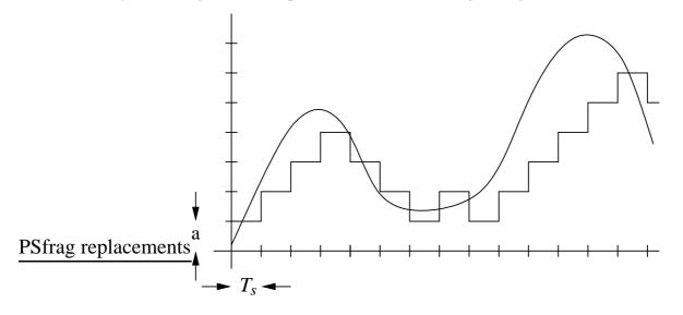
The signal is first quantised into discrete levels, but the size of the step between adjacent samples is kept constant. The signal may therefore only make a transition from one level to an adjacent one. Once the quantisation operation is performed, transmission of the signal can be achieved by sending a zero for a negative transition, and a one for a positive transition. Note that this means that the quantised signal *must* change at each sampling point.
