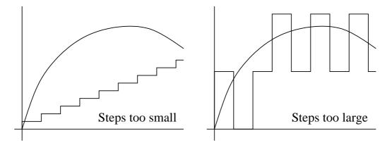
If the signal has a known upper-frequency cutoff  $\omega_m$ , then we can estimate the fastest rate at which it can change. Assuming that the signal is  $f(t) = b \cos(\omega_m t)$ , the maximum slope is given by
