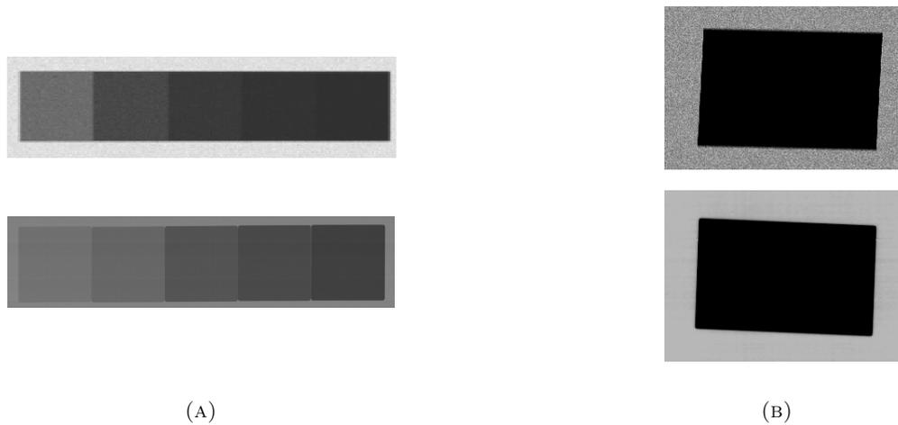
FIGURE 5.10: The simulated (top) and real (bottom) X-ray images of the (A) aluminium and (B) tungsten test objects. The tungsten test object is at a slight angle (less than 2 degrees) to the detector for the DQE calculation.
