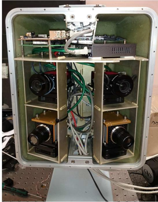
Figure 6.2: Inner camera array assembly of System 1.
