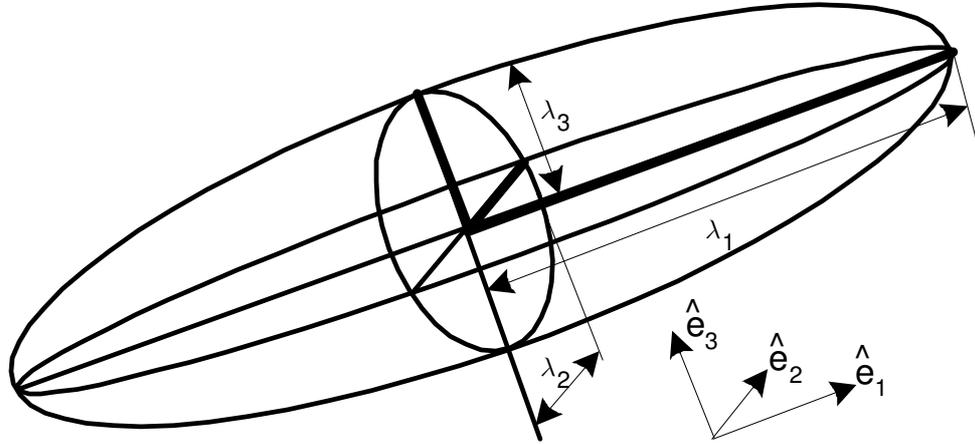
Figure 2.8: 3D ellipsoid tensor representation.
