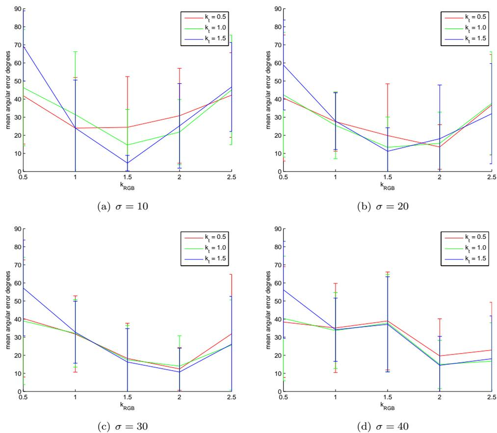
Figure 5.11: Error bars on the average angular errors on the *Flower Garden* sequence tree trunk (case 6, pre-alignment voting) for various  $k_t$ ,  $k_{RGB}$  and  $\sigma$ . The parameter  $k_{xy} = 1$ .
