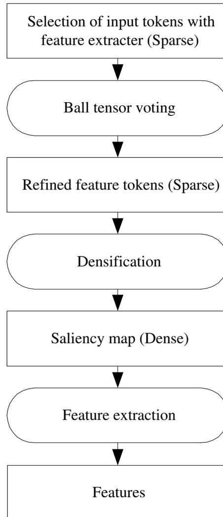
Figure 2.13: Generalised tensor voting flow diagram.
