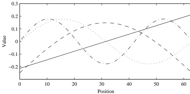
Figure 5.3: Nonorthogonal basis functions for invariance subspace.
