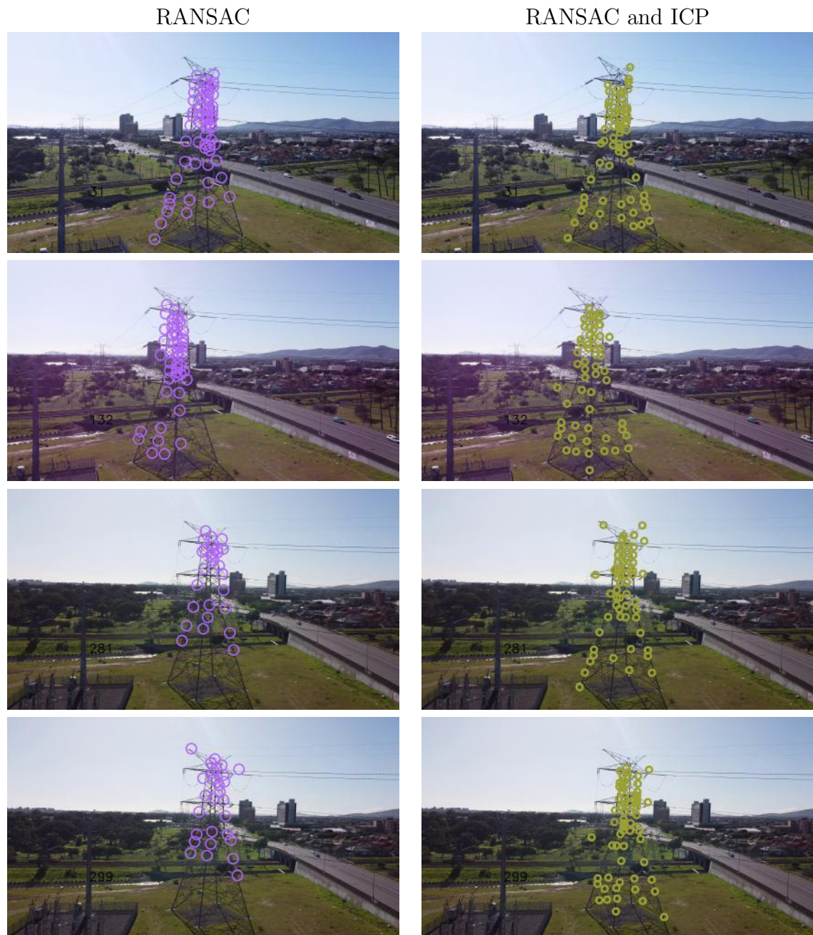
FIGURE 6.27: Results of the 3D model of the pylon registering onto the image of the pylon with RANSAC as a means of data association.
