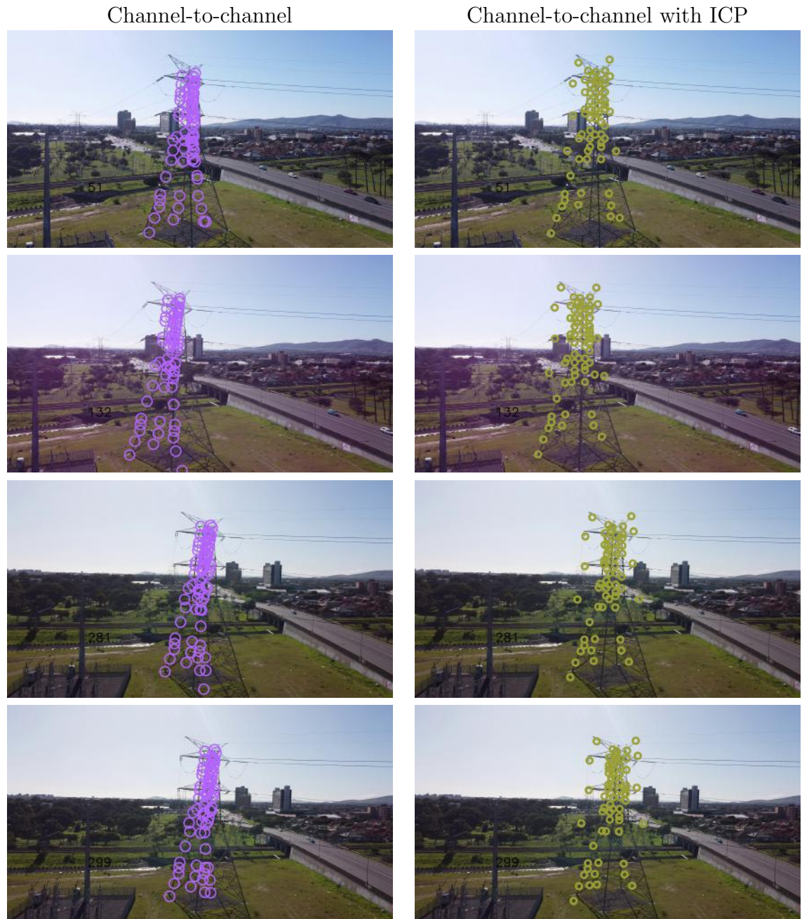
FIGURE 6.26: Results of the 3D model of the pylon registering onto the image of the pylon with channel-to-channel as the means for data association .
