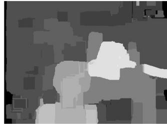
(b) Disparity map produced by using the SSD algorithm.
