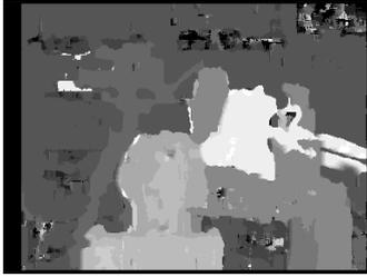
(c) Disparity map produced by using the sum of absolute differences with a  $9 \times 9$  window of absolute differences with a  $9 \times 9$  window size.
