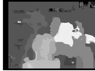
(d) Disparity map produced by using the sum of absolute differences with a  $15 \times 15$  window size.
