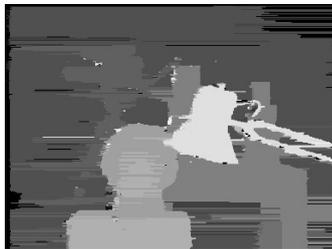
(c) Disparity map produced by using the DP algorithm.
