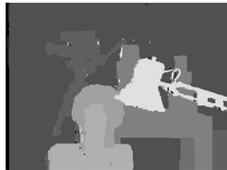
(d) Disparity map produced by using the GC algorithm.
