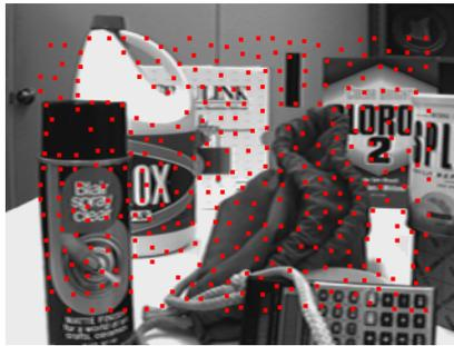
Figure 5.1: Features detected in the image. 313 KLT features are detected on this image.
