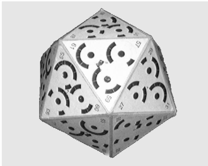
Figure 1.4: Calibration object for the VCAL calibration software.
