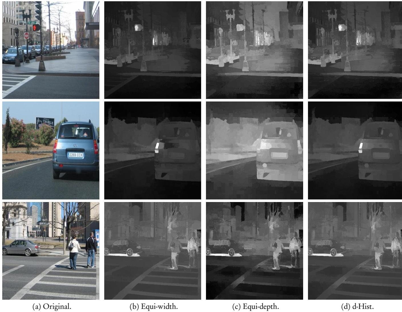
Figure 3.5.3: Example images and their saliency maps computed with different histogram construction methods.
