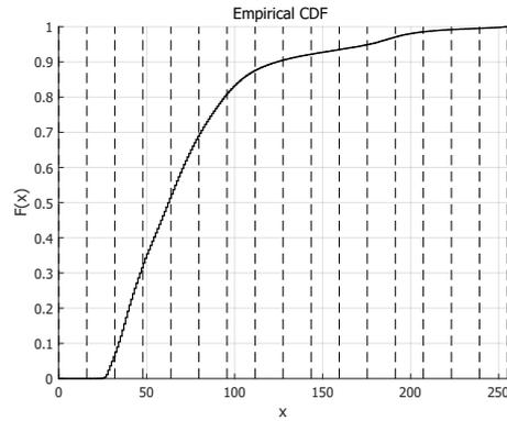
(b) Partitioning the domain of the ecdf generates the equi-width histogram.
