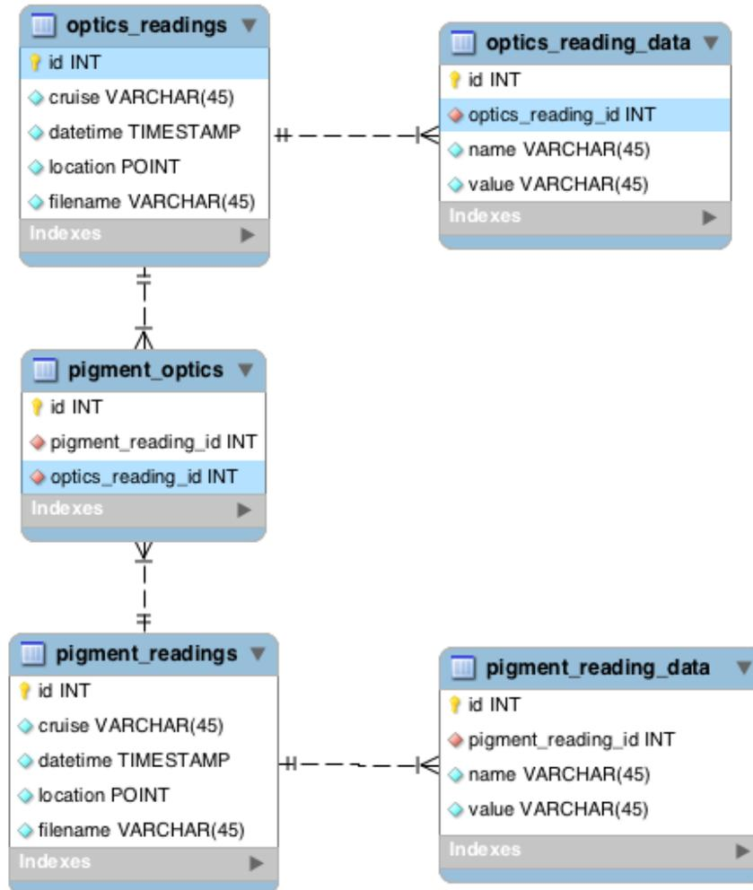
Figure 16: Tara database ERD for storing absorption and pigment data.
